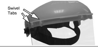
2. Engage the visor with the swivel tab at the front. Slide the visor slots onto the four swivel tabs and turn to secure the visor. Replace visor fixing nuts.
