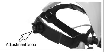
The headband should be adjusted to fit the wearer's head. To do this, turn the adjustment knob either left or right to expand or contract the headband.
